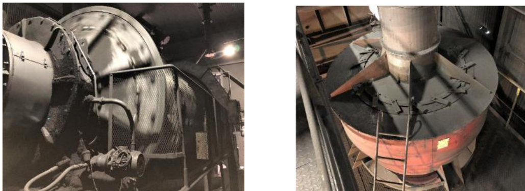
Figure 3. Ball mill and static classifier at AoG.
